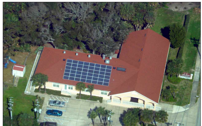
The UU Society of the Daytona Beach Area's photovoltaic panels. This system produces 10kw of energy for the church's use.
